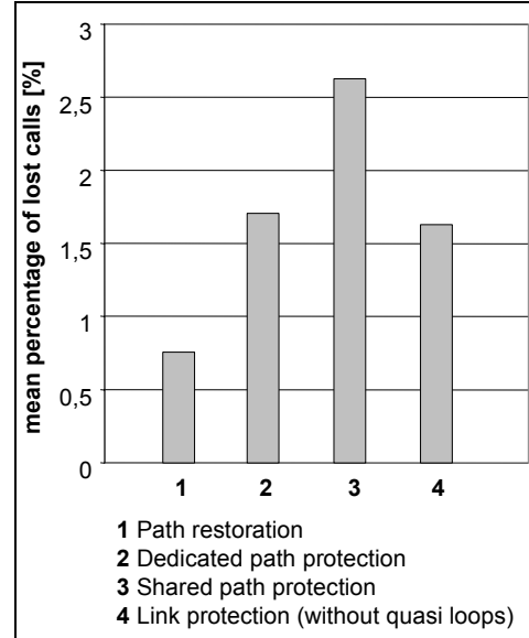
Figure 12: Mean percentage of lost calls in case of double failures in a transparent network
